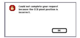
The CCD pixel position value may become corrupted as the result of a power surge or power failure. If this occurs, you must enter the correct value before starting the run. For details, refer to the ABI PRISM 377 DNA Sequencer User's Manual.
